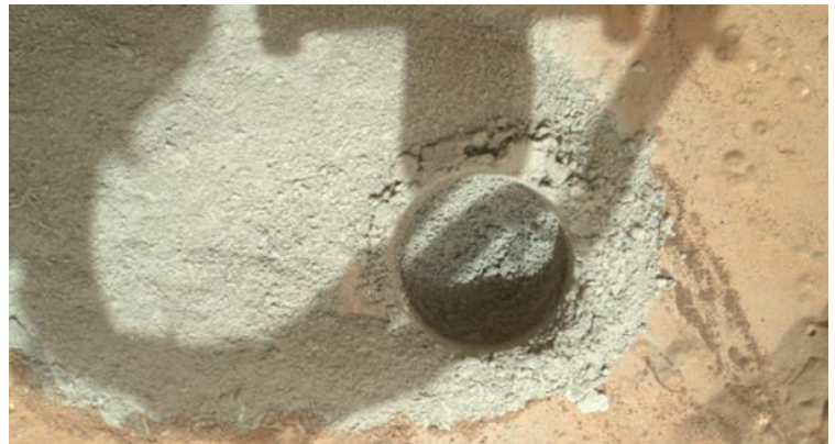
Preparatory Test of Drilling on Mars Generates Rock Powder: Image Credit: NASA/JPL-Caltech/MSSS
