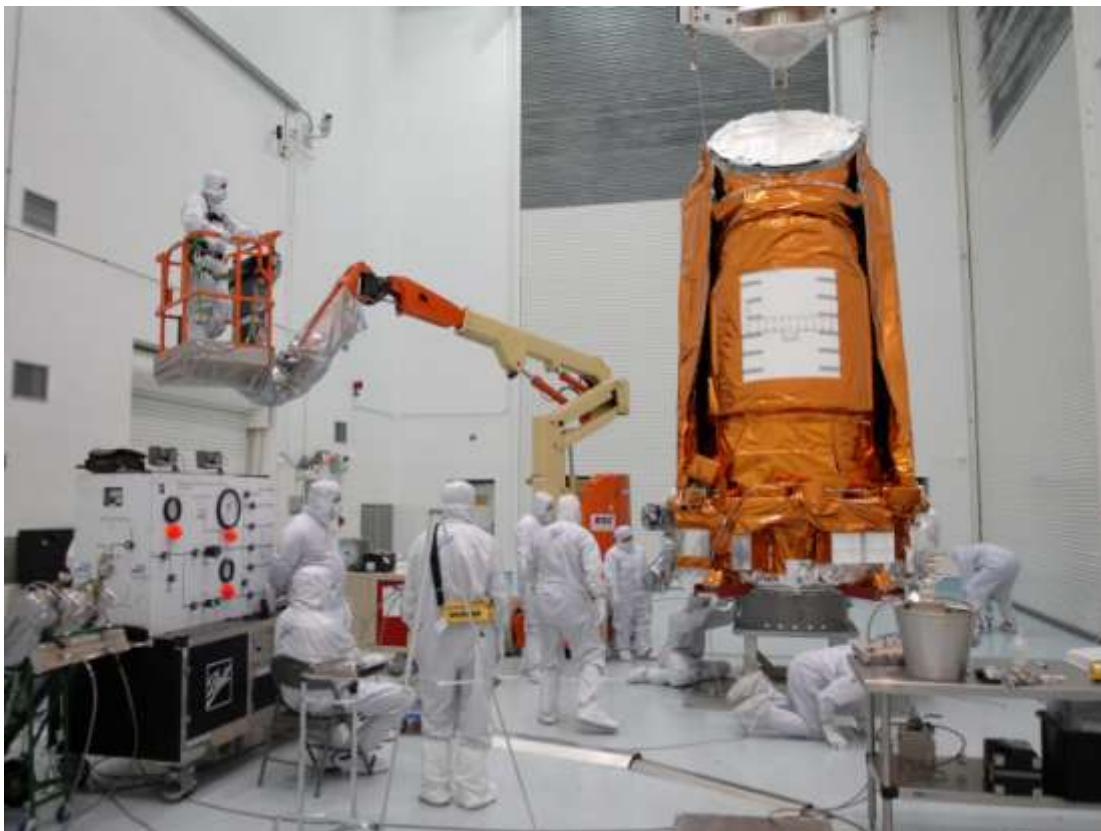
Above: Kepler on the stand in Cape Canaveral being fueled up. Kepler is the pioneering space craft in the search for extrasolar planets. Image credit: NASA
