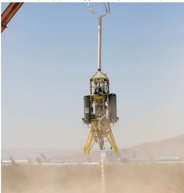
Tethered test flight of Masten's XA-0.1B Image courtesy of Masten Space Systems, Inc.
